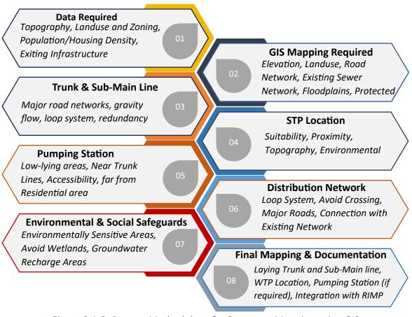
Figure 3.1-2: Process Methodology for Sewerage Mapping using GIS
