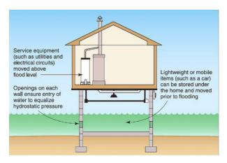
Figure 3.4-1: Elevated structure design for flood risk area
