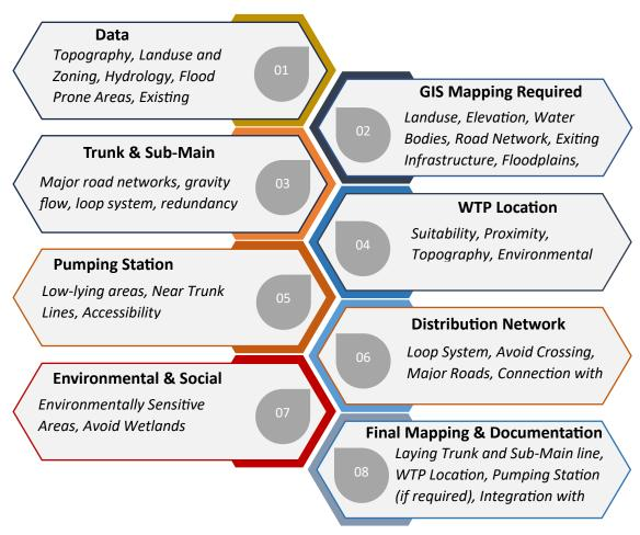
Figure 3.1-1: Process Methodology for Water Supply Mapping using GIS
