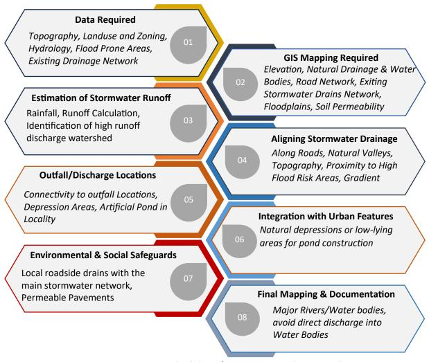
Figure 3.3-1: Process methodology for stormwater drainage planning
