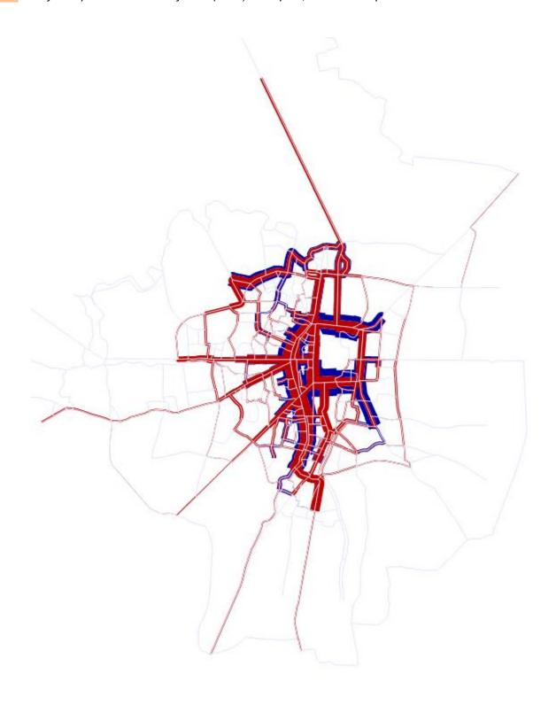
Figure 9-1 Peak Hour PCU assignment of BAU Scenario (Peak Hour – HY2044)
